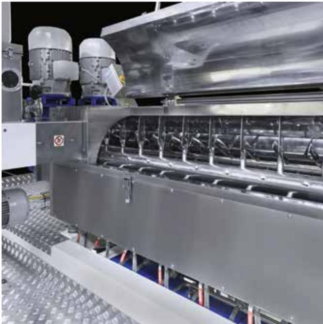
Detail of a TT92 cooking extruder steaming tank and the characteristic paddle shaft.
