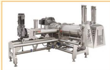
The **EX Continuous Mixer** produces low absorption dough for products such as sweet goods, crackers, and pet treats, and is also well suited for all but the lowest viscosity powder/liquid mixtures.
