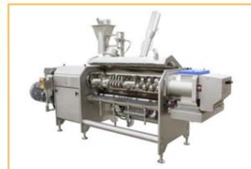
The **LDX Continuous Mixer** combines all ingredients except flour in the creme up stage. In the first stage, special mixing elements cut the fat into the other ingredients. The flour is added before the development stage where the final dough is created. This mixer is ideal for most types of cookies or any application where ingredients are blended before the flour is added.
