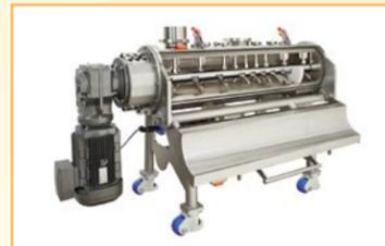
The **FX Continuous Mixer** is a high intensity mixer that produces dough typically used for wheat, potato, corn masa flour and multi-grain snack products.
