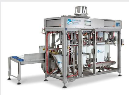
*OmniStar with a duplex MasterWeigh 60-series scale can run up to 20 bags/min.*
