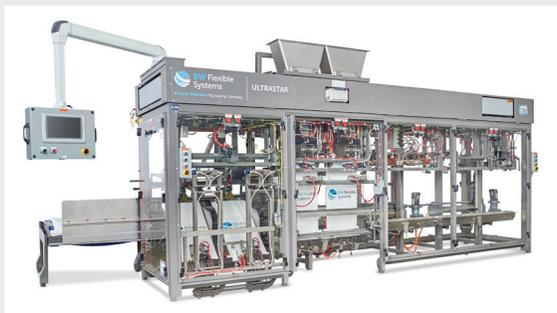
*UltraStar with its quad MasterWeigh 60-series scales can run up to 38 bags/min.*
