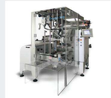
*Hayssen DoyZip 380 -VFFS for pillow, gusseted, block-bottom, quad four-corner seal, three-side seal or Doy bag, with or without zip close.*
