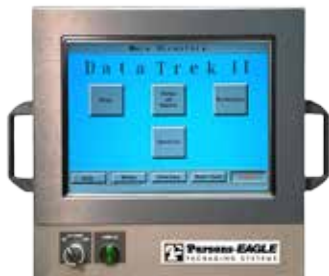
Operator Interface Terminal
